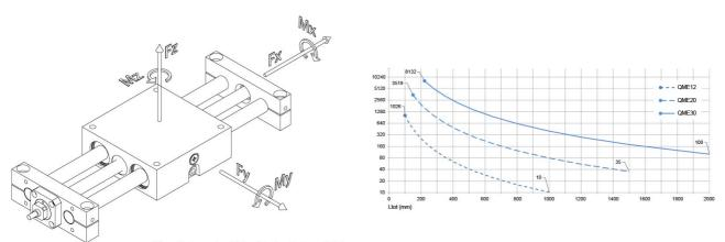
\*All capacity values are theorethical maximal values without any safety factor. Permissible load depends on desired life time and/or permissible deflection of the shafts. For motor driven units in automation applications, a dynamic safety factor of at least 5 is recommended.
