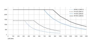
\* All capacity values are theorethical maximal values without any safety factor. Permissible load depends on desired life time and/or permissible deflection of the shafts. For motor driven units in automation applications, a dynamic safety factor of at least 5 is recommended.
