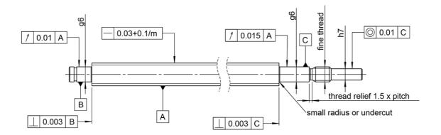
Recommended dimensional and geometrical tolerances for typical machining of miniature ball screws. Undercuts, radii and thread reliefs to be checked for suitability for chosen bearing- and lock-nut solution.
