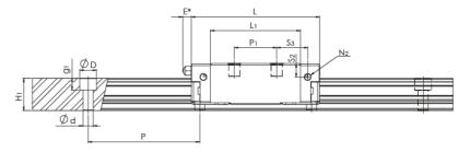
\*Size 21/15 delivered with straight standard nipple. Size 27/20 delivered with angled standard nipple.
