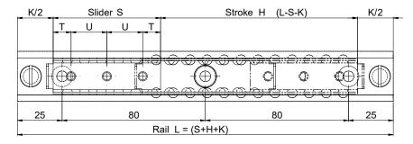
Note: To ensure that all fixing holes of the rail are accessible, S must be < L/2 - K. To ensure proper smooth movement it is necessary that H  $\le$  7S
