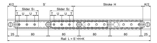
Version 3 is a variant of version 1 with several synchronized sliders. The total load capacity is based on the number of sliders in the rail. The length of the individual sliders can therefore vary.
