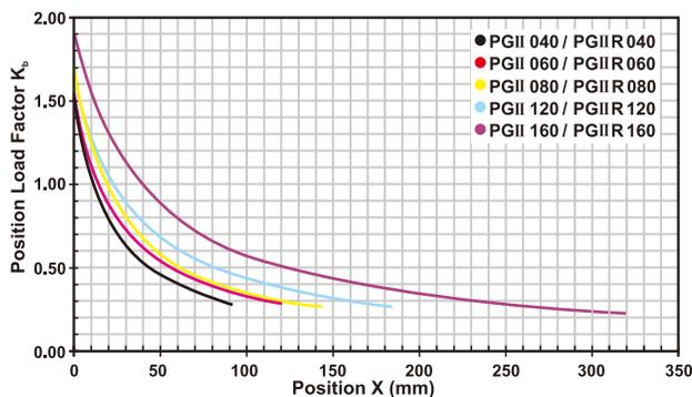
If radial force  $F_{2r}$  is not exerted on the center of the output shaft  $X < 1/2 L$  or  $X > 1/2 L$ , the permitted radial and axial loads can be calculated by the position load factor  $K_b$  on the above diagram.
