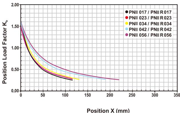
If radial force  $F_{2r}$  is not exerted on the center of the output shaft  $X < 1/2xL$  or  $X > 1/2xL$ , the permitted radial and axial loads can be calculated by the position load factor  $K_b$  on the above diagram.
