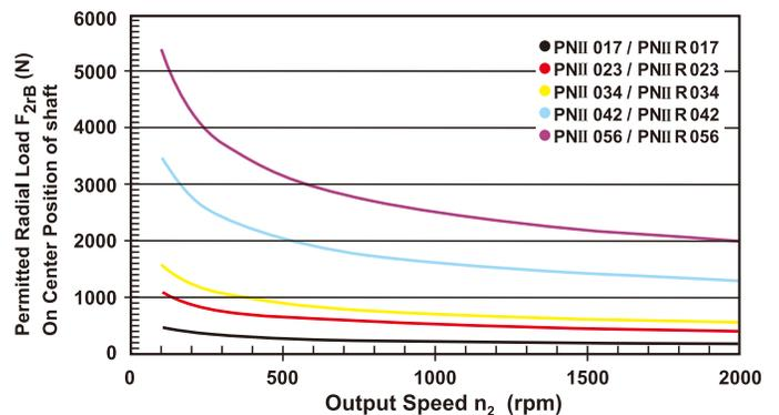
Permitted radial load  $F_{2r}$  on center of output shaft  $X = 1/2 \times L$  for various output speeds. Values provided are for 20,000 hours<sup>(C)</sup> life.
