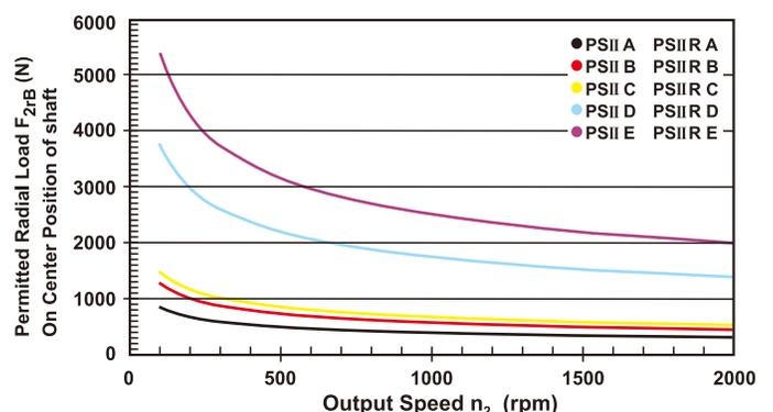
Permitted radial load  $F_{2r}$  on center of output shaft  $X = 1/2 L$  for various output speeds. Values provided are for 20,000 hours<sup>(C)</sup> life.
